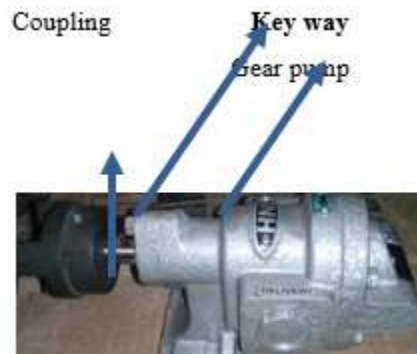
Fig : 4.1-Keyway on shaft of gear pump
